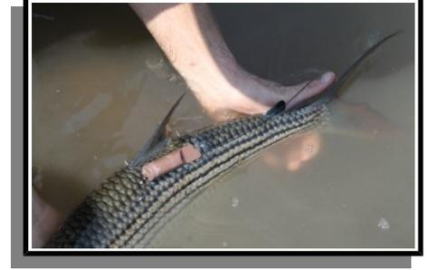
The WW0500AS-aquatic transmits **and stores** location and behaviour information periodically, according to an established scenario (user defined schedule), when a defined violation of “normal” behaviour is observed or on request from the user. This data is received in real time by a base station located within range of the tagged animals or the data is downloaded when the animal enters a coverage area.
